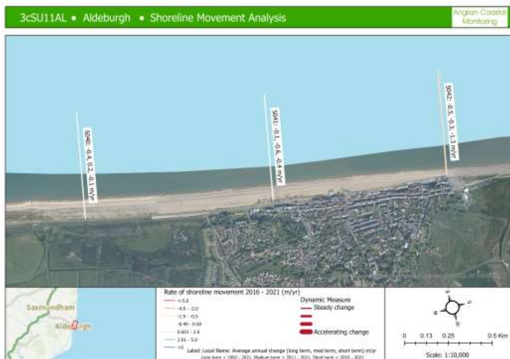
Figure 1: Missing figure from the ACMP's Suffolk (SMP 7) Coastal Trends Report 2021. Figure shows rates of Shoreline Movement (at Mean Sea Level) for the Aldeburgh monitoring cell.
